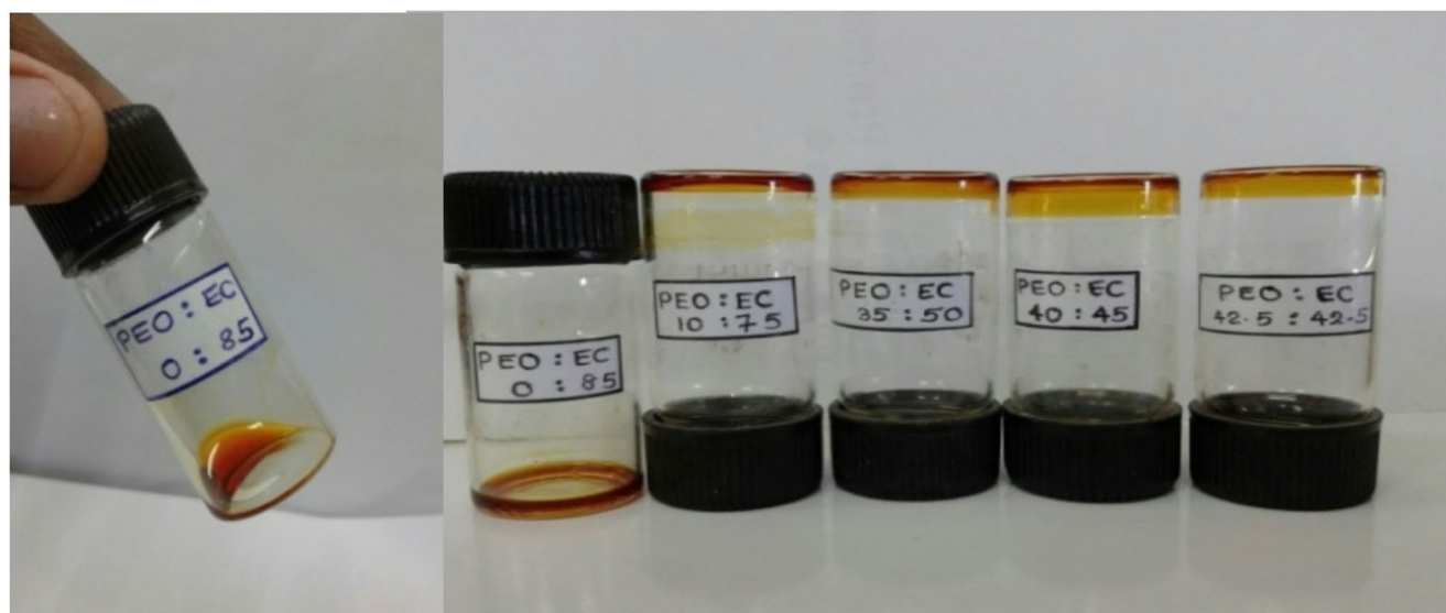
Fig. 1 The inverted bottle test; The solid nature of the electrolytes PEO: EC: \text{Pr}_4\text{N}^+\text{I}^-:\text{I}_2 after 4 h of vacuum drying at room temperature. PEO: EC weight ratios 10:75, 35:50, 40:45, 42.5:42.5, and 75:10 w/w% and the liquid nature of PEO: EC=0:85 w/w% (PEO-free) electrolyte
