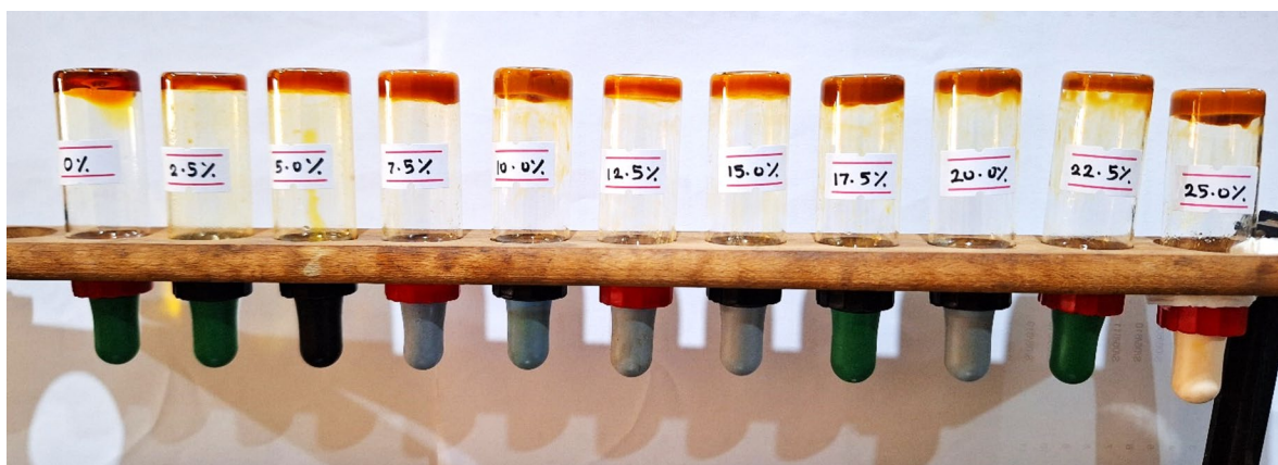
Fig. 2 The gel-polymer electrolyte series varying added \text{TiO}_2 percentage from 0.0–25.0%
