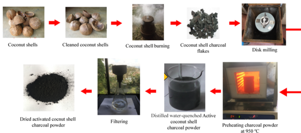
Figure 1. Process used to prepare coconut shell-based activated carbon.
