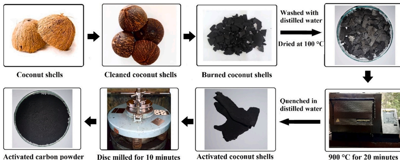
Fig. 2. Schematic diagram of the process of making activated carbon powder from coconut shells.
