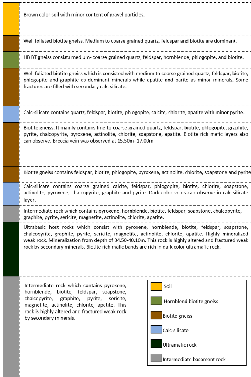
Fig. 4. Macroscopic observations of the borehole core with log data.
