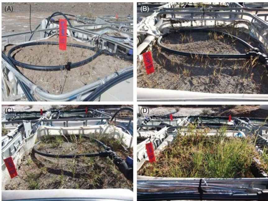
Figure 4 The emergence and growth of mixed grass species in (A) intact tailings (B) loose tailings (C) tailings amended with 10% hay (v/v) and (D) tailings amended with 20% hay (v/v). The surface of the tailings was covered with a layer of black soil (about 10 cm), into which mixed grass species were sown on Jan. 18, 2011. The photos were taken on Apr. 10, 2011 (Huang et al., 2011).
