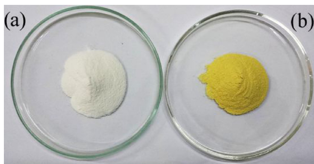
Fig. 3. (a) Undoped TiO 2 powder in white colour (left) and (b) N-doped TiO 2 powder in yellowish colour prepared in this work.
