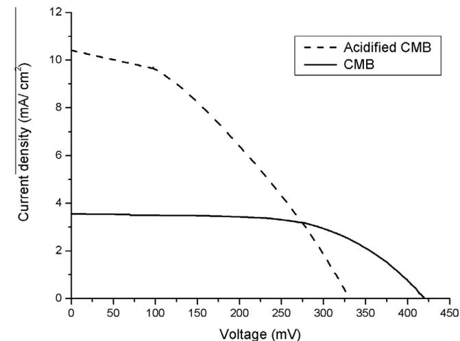
**Fig. 6.** Comparison of current voltage ( $I$ - $V$ ) characteristics of DSSCs sensitized with CMB dye (with and without acidification).
