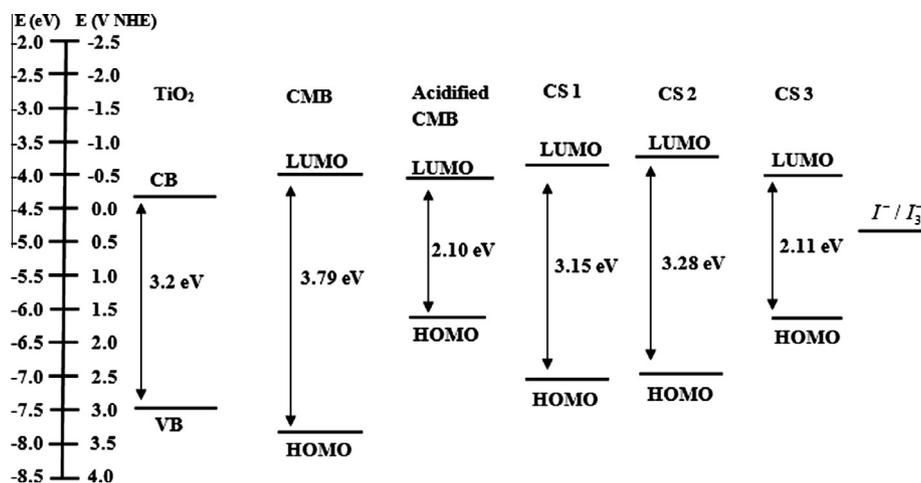
Fig. 8. Schematic diagram showing the calculated positions of HOMO and LUMO levels of the investigated dye pigments with respect to the vacuum level and NHE.
