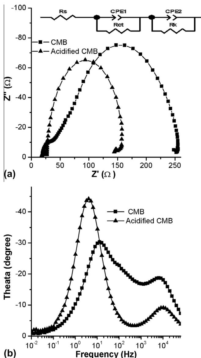
Fig. 9. Electrochemical impedance spectra measured under the illumination ( $100 \text{ mW cm}^{-2}$ ) and open circuit conditions for DSSCs sensitized with CMB and acidified CMB. (a) Nyquist plots. (b) Bode phase plot. Inset of (a) shows the equivalent circuit diagram for EIS.
