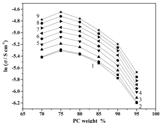
**Fig. 2** Variation of the conductivity with PC concentration (by weight %) at different temperatures (1: 25 °C, 2: 30 °C, 3: 35 °C, 4: 40 °C, 5: 45 °C, 6: 50 °C, 7: 55 °C, 8: 60 °C, 9: 65 °C)
