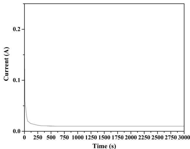
**Fig. 4** DC polarization curve taken with configuration SS/NCPE/SS under 1.0 V DC voltage. SS stainless steel
