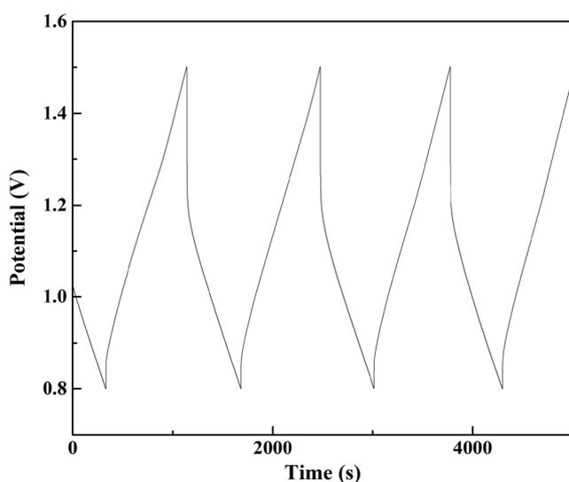
**Fig. 8** Variation of discharge capacity of the redox capacitor upon continuous charging and discharging under a constant current of  $10 \mu\text{A}$
