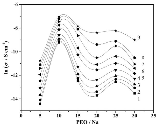
**Fig. 1** Variation of the conductivity of the PEO/ $\text{NaClO}_4$  polymer electrolyte with PEO/ $\text{NaClO}_4$  molar ratio at different temperatures (1: 25 °C, 2: 30 °C, 3: 35 °C, 4: 40 °C, 5: 45 °C, 6: 50 °C, 7: 55 °C, 8: 60 °C, 9: 65 °C)
