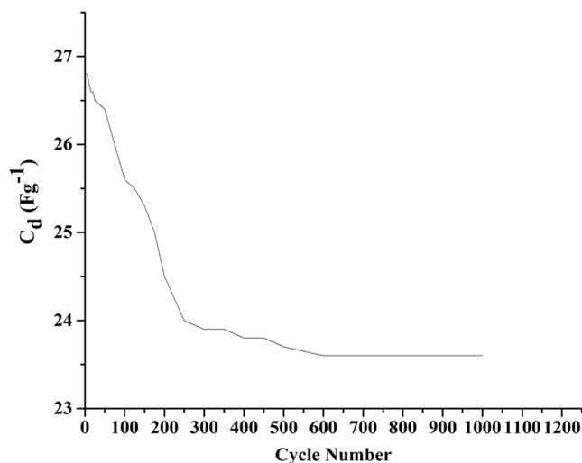
**Fig. 9** Variation of discharge capacity of the redox capacitor upon continuous cycling
