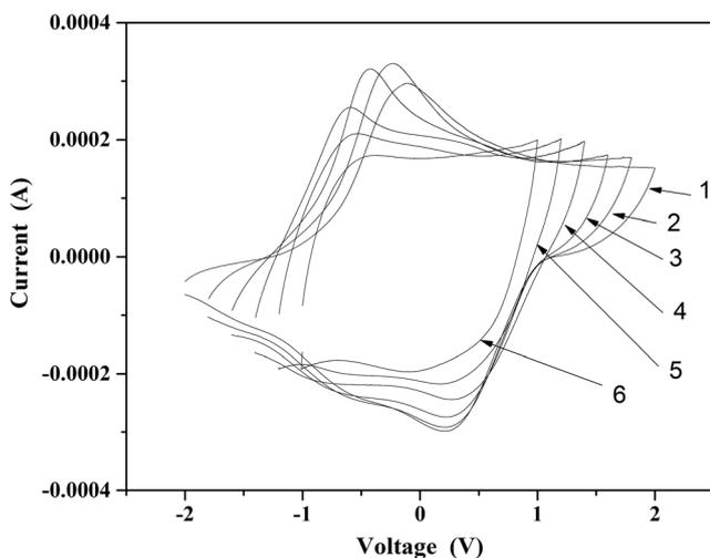
**Fig. 5** Cyclic Voltammograms obtained for the redox capacitor, PPy: NCPE: PPy at different potential windows (1:  $-2$  to  $2 \text{ V}$ , 2:  $-1.8$  to  $1.8 \text{ V}$ , 3:  $-1.6$  to  $1.6 \text{ V}$ , 4:  $-1.4$  to  $1.4 \text{ V}$ , 5:  $-1.2$  to  $1.2 \text{ V}$ , 6:  $-1.0$  to  $1.0 \text{ V}$ )
