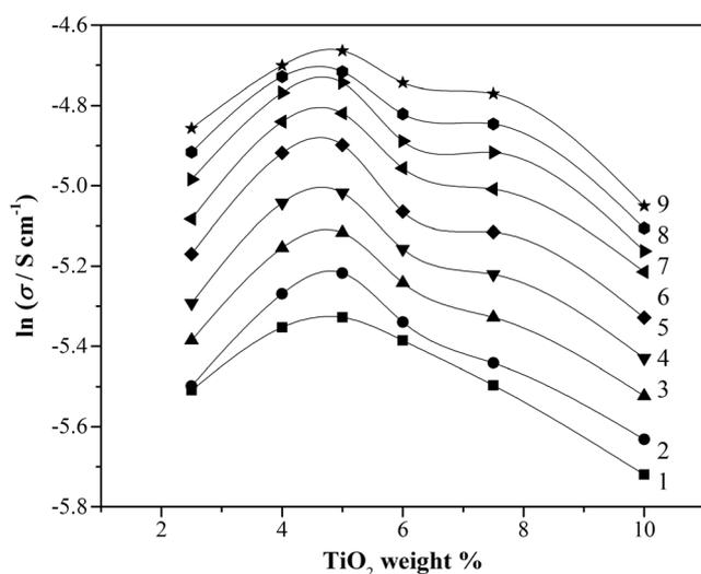
**Fig. 3** Variation of the conductivity with  $\text{TiO}_2$  concentration (by weight %) at different temperatures (1: 25 °C, 2: 30 °C, 3: 35 °C, 4: 40 °C, 5: 45 °C, 6: 50 °C, 7: 55 °C, 8: 60 °C, 9: 65 °C)
