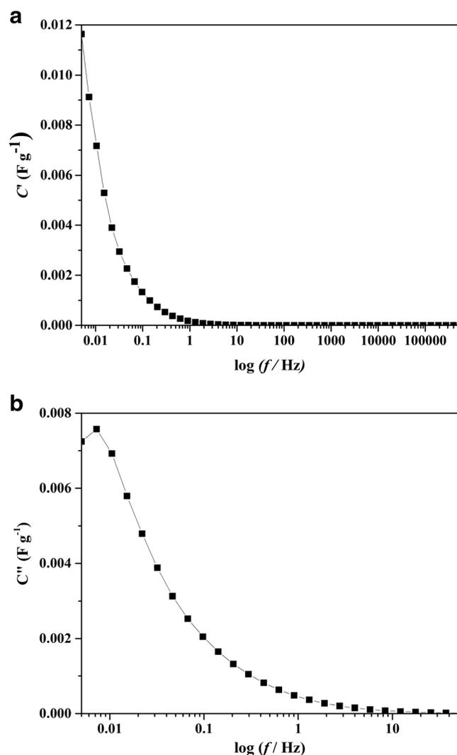
**Fig. 6** a, b Bode plots drawn as real capacitance versus frequency and imaginary capacitance versus frequency, respectively
