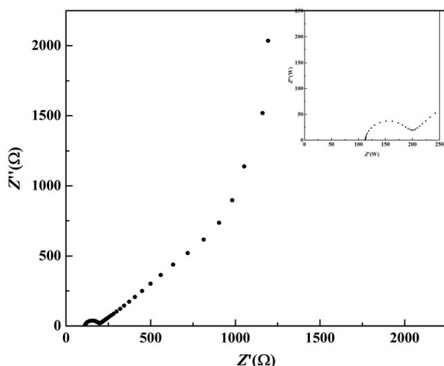
**Fig. 7** Resulting Nyquist plot of the redox capacitor, PPy: NCPE: PPy (Inset: expanded area at high-frequency range)
