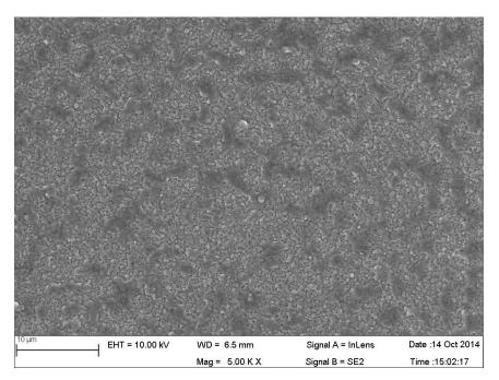
Figure 1: SEM image of the TiO<sub>2</sub> spin-coated layer (the 1<sup>st</sup> layer) prepared on FTO substrate.
