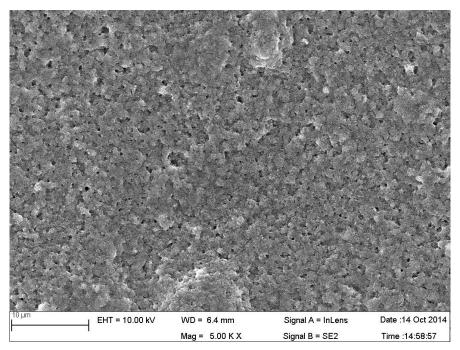
**Figure 2:** SEM images of the  $TiO_2$  film prepared using Doctor blade method (the 2<sup>nd</sup> layer) prepared on the spin coated layer.
