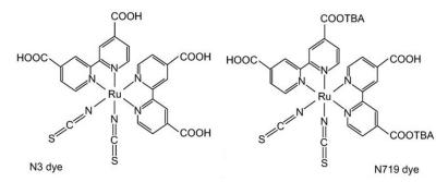
**Figure 6:** The structure of N3 (cis-Bis(isothiocyanato) bis(2,2'-bipyridyl-4,4'-dicarboxylato ruthenium(II)) and N719 (Ditetrabutylammonium cis-bis(isothiocyanato)bis(2,2'-bipyridyl-4,4'-dicarboxylato)ruthenium(II)) dye sensitizers. (TBA=tetra-butylammonium)
