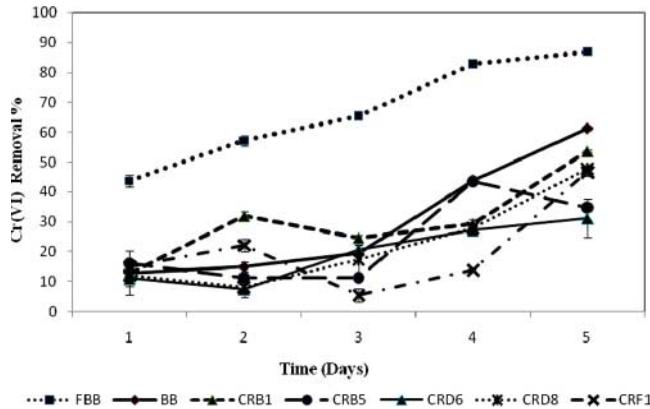
Figure 4. Cr(VI) removal over time by FBB, BBs and bacterial isolates (CRD 6, CRD 8, CRB 1, CRB 5). The initial concentration was  $100 \mu\text{g mL}^{-1}$  Cr(VI). Different letters at each time show significant differences at 5% probability, whereas the absence of letters indicates absence of significant differences at the same probability level. Vertical bars show standard errors.
