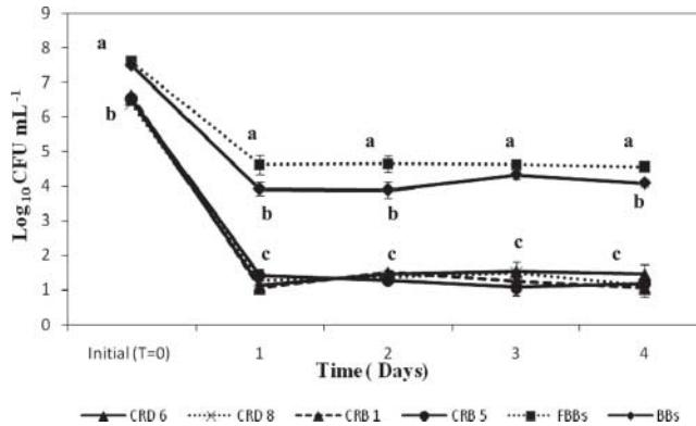
Figure 2. Change in CFU of bacterial isolates (CRD 6, CRD 8, CRB 1, CRB 5) and biofilms (FBBs and BBs) against different Cr(VI) concentrations after 24 h incubation. Different letters in each concentration show significant differences at 5% probability, whereas the absence of letters indicates the absence of significant differences at the same probability level. Vertical bars show standard errors.
