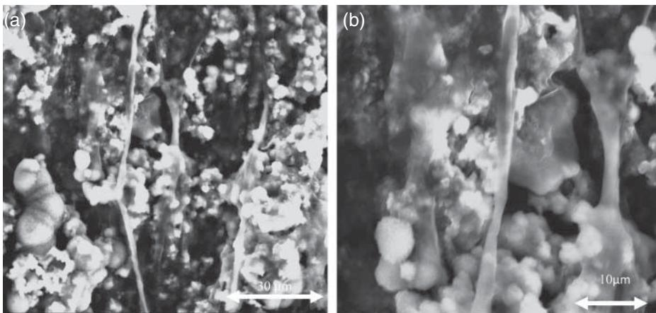
Figure 5. SEM images of FBBs. Extensive EPS covering of FBBs can be seen. The scale bar represents 30 and 10  $\mu\text{m}$ , respectively.
