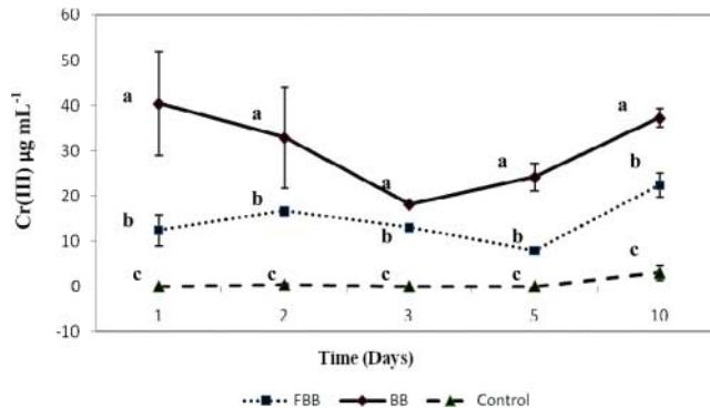
Figure 7. Cr(III) concentration in the bioreactor over time by FBBs and glass-wool-attached BBs. Different letters at each time show significant differences at 5% probability. Vertical bars show standard errors.
