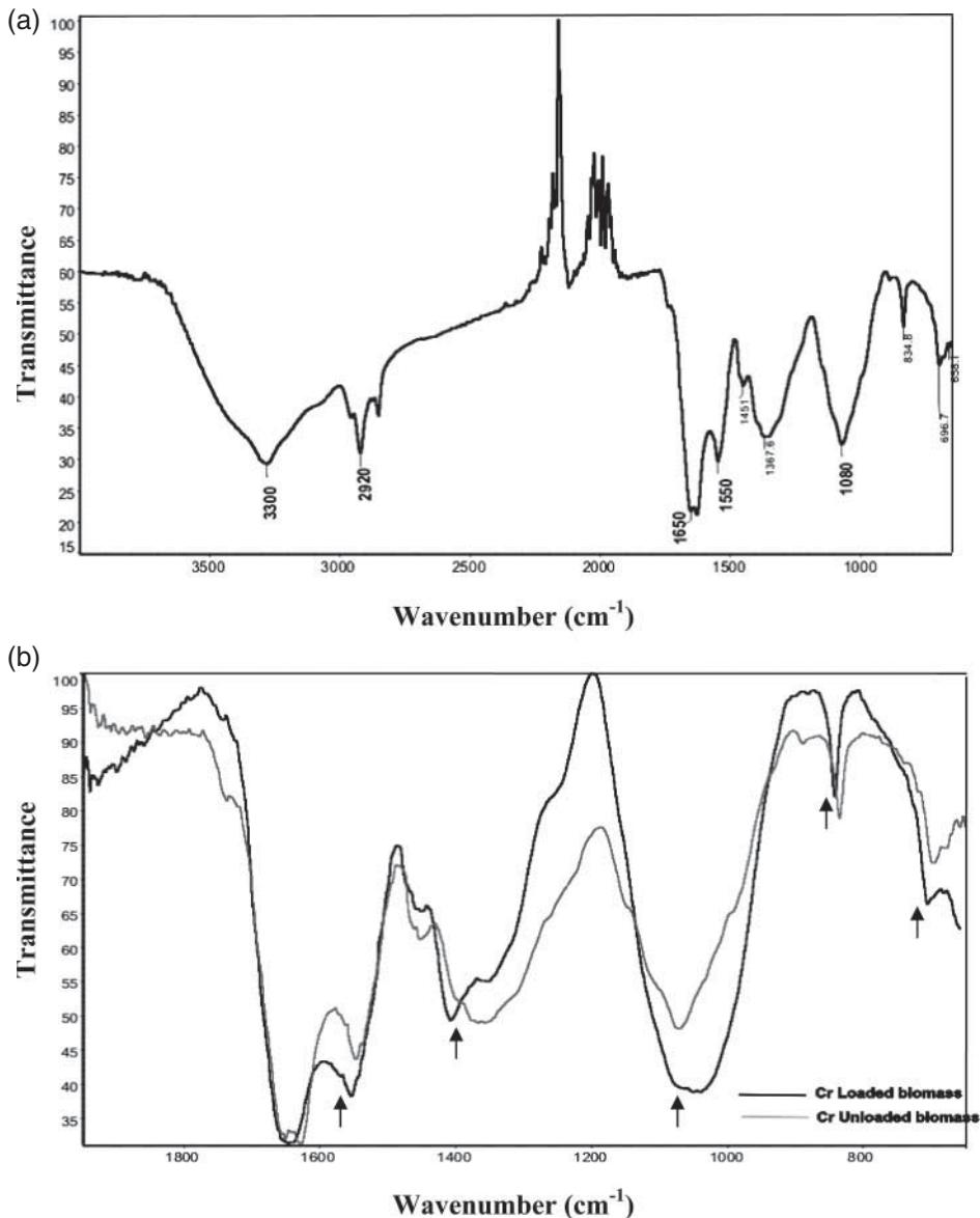
Figure 8. (A) FT-IR spectrum of FBB before Cr(VI) loading. (B) Highlighted view of wavenumber range 800–1800 cm<sup>-1</sup> of FBB before and after Cr(VI) loading. Black arrows indicate spectral pattern shifting of certain bands observed in the spectrum.
