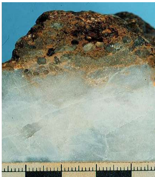
Figure 2. Partially weathered carbonatite rock with small primary apatite crystals (pale green), dissolution cavities and partially developed secondary material (brown colour). Width of the photograph is about 11 cm.
