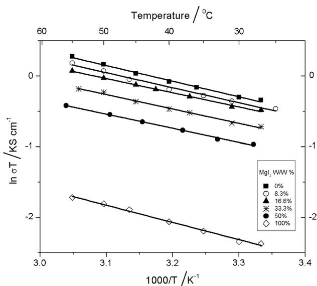
**Fig. 2** The variation of  $\ln \sigma T$  plotted against the reciprocal absolute temperature for PAN/EC/PC/MgI<sub>2</sub>/Pr<sub>4</sub>NI/I<sub>2</sub> gel electrolytes containing different MgI<sub>2</sub>/Pr<sub>4</sub>NI ratios
