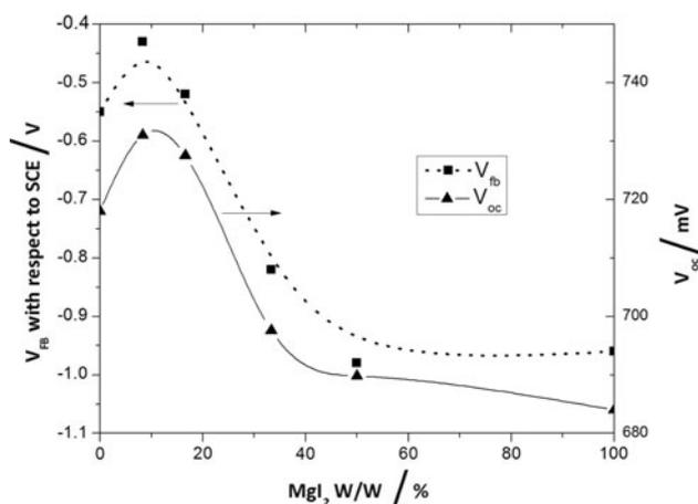
**Fig. 6** Variation of the flat-band potential ( $V_{fb}$ ) with wt%  $MgI_2$  for the  $TiO_2$  electrode immersed in the solution electrolyte EC/PC/ $MgI_2$ / $Pr_4NI$ . Variation of the open circuit photovoltage ( $V_{oc}$ ) of the DSSC with PAN/EC/PC/ $MgI_2$ / $Pr_4NI/I_2$  gel electrolyte is also shown for comparison
