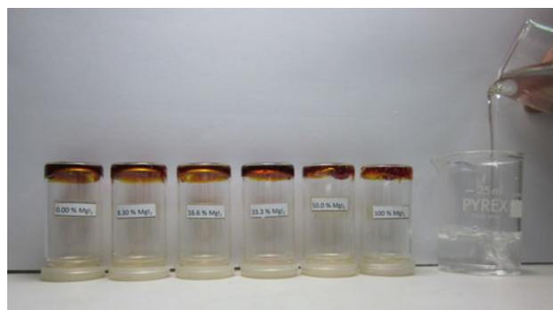
**Fig. 1** The six gel electrolyte samples prepared with different  $\text{MgI}_2/\text{Pr}_4\text{NI}$  weight ratios in “inverted” sample bottles to show the gel nature of the electrolytes. From left to right, the  $\text{MgI}_2$  wt% are: 0, 8.3, 16.6, 33.3, 50, 100
