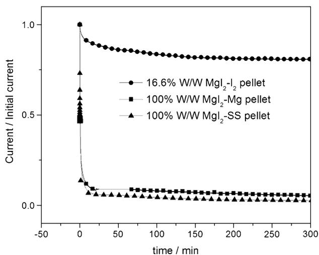
**Fig. 3** Current/initial current versus time plots for the some selected electrolyte samples obtained by DC polarization test with iodine non-blocking electrodes, Mg non-blocking electrodes, and stainless steel blocking electrodes
