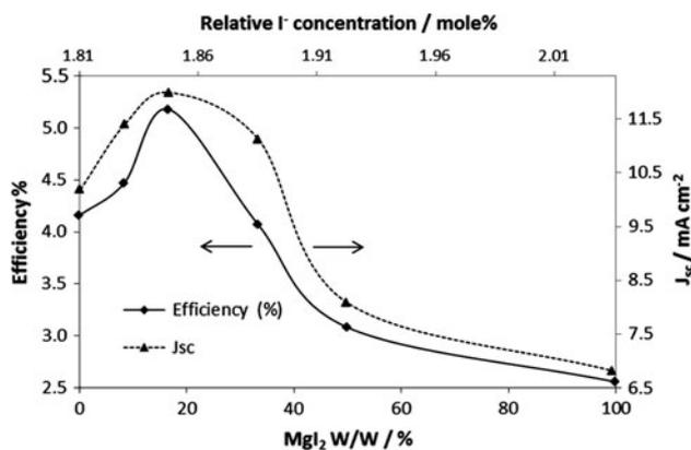
**Fig. 5** The variation of (*thin line*) the efficiency ( $\eta$ ) and (*dotted line*) the short circuit photo current density ( $J_{sc}$ ) of all six solar cells as a function of the wt%  $MgI_2$
