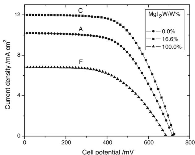
**Fig. 4** The photocurrent–photovoltage ( $I$ – $V$ ) characteristics of three solar cells where the gel electrolyte salt compositions are: (A) 0 wt%  $\text{MgI}_2$  (only  $\text{Pr}_4\text{NI}$ ) (C) 16.6 wt%  $\text{MgI}_2$  + 83.4 wt%  $\text{Pr}_4\text{NI}$  and (F) 100 %  $\text{MgI}_2$ . (100  $\text{mW cm}^{-2}$ , A.M. 1.5, active area  $0.25 \text{ cm}^{-2}$ )
