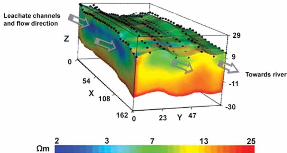
Figure 7. Three-dimensional cube synthesized from 2D imaging profile (a–h) obtained from the dumpsite. The section normal to y-axis and normal to z-axis indicates the flow patterns. The sections normal to z-axis reveal that the leachate flow is limited to around 10-m level.
