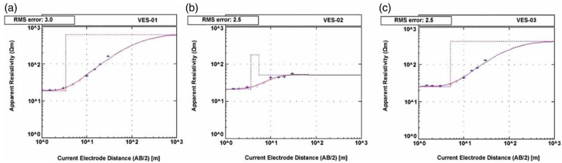
Figure 3. Vertical electrode sounding (VES) interpretation with true resistivity values. The subparts (a), (b) and (c) are related to the VES-01, VES-02 and VES-03, respectively (values are elaborated in Table 1).
