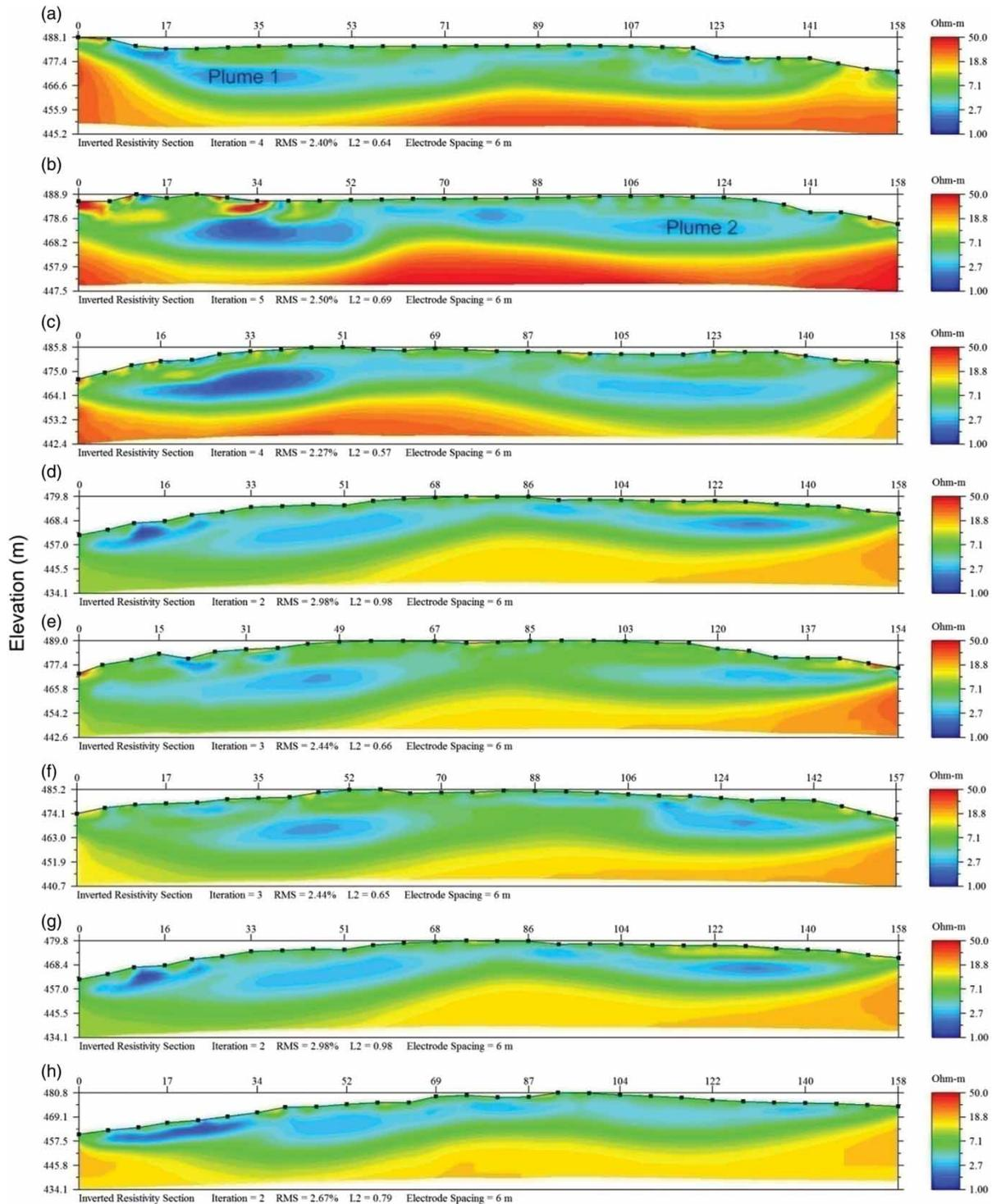
Figure 6. (a–h) Resistivity profile images along the profile line-01 to line-08, respectively, on the dumpsite. Data were acquired at 2.5-m electrode interval with 158-m total spread.
