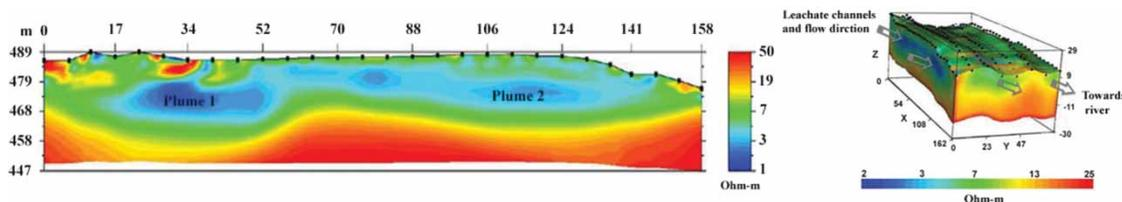
**Keywords:** resistivity techniques; electrical conductivity; municipal solid waste dumpsites; leachate plume delineation; Sri Lanka
