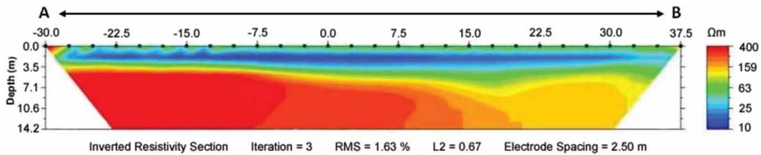
Figure 4. Resistivity image along the profile line-06. Data were acquired at 2.5-m electrode interval with 67.5-m total spread. The resistivity range is set at 400 and 10  $\Omega\text{m}$  maxima and minima and 400  $\Omega\text{m}$  is set as the lowest value for bedrock (partially weathered rocks).
