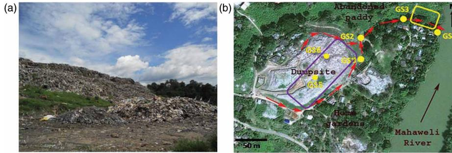
Figure 1. (a) View of the Gohagoda open solid waste dumpsite. (b) Schematic diagram of the leachate drainage channel (red arrows), leachate sampling points (yellow dots) and resistivity data acquisition area (yellow and purple rectangles for phases 1 and 2, respectively) at Gohagoda dumpsite.
