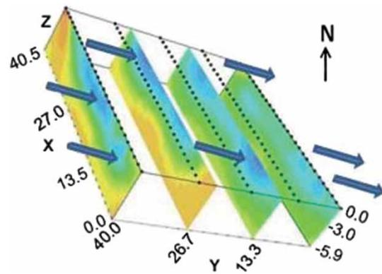
Figure 5. Two-dimensional imaging profile at leachate-contaminated area at Gohagoda dumpsite. Sliced section normal to y-axis and normal to z-axis indicates the flow patterns. The sections normal to z-axis reveal that the leachate flow is at very shallow level and limited to 3-m level. Blue arrow shows the leachate flow direction towards the river.
