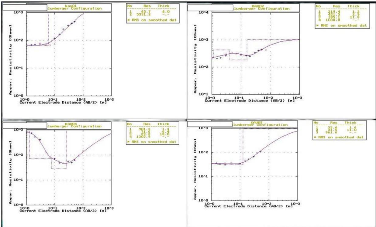
**Fig. 6.** Vertical Electrical Sounding (VES) plots for the study site. Top left; VES01 (256205 N, 166759 E), top right; VES 02 (256212 N, 166641 E), lower left; VES03 (256224 N, 166524E), lower right; VES04 (256632 N, 166648 E).
