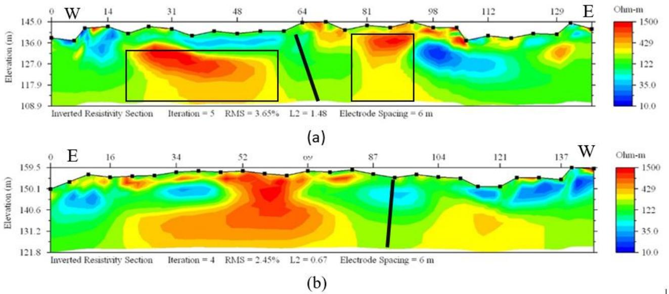
**Fig. 4.** Resistivity profiles of area 1. The top figure is profile 2D1 and the one at the bottom is 2D2. The black rectangles show the magnetite containing weathered bed rock. The near vertical dark lines are the weak zones.
