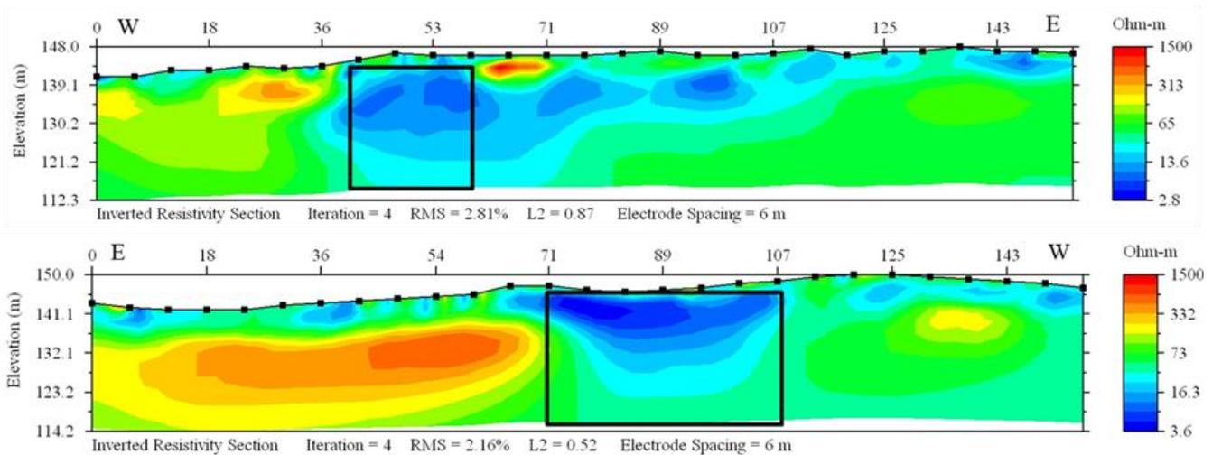
**Fig.5.** 2D profiles of area 2. The top figure is 2D3 profile and the bottom one is 2D4. In these diagrams the dark rectangles show very low resistive areas at some locations extending to depths of about 20 m.
