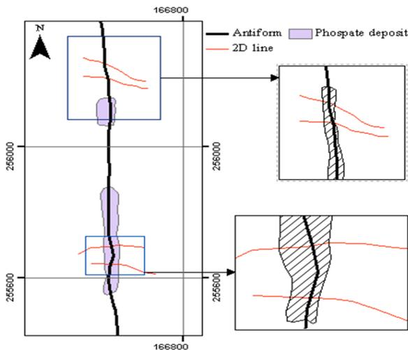
**Fig. 07.** Location of phosphate deposit and antiform with weak zones identified in resistivity profiling. The first and the last electrode of the 2D lines have been extended (dashed lines) to demarcate the weak zone along the axis of the antiform.
