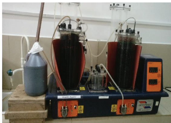
Figure 3 – Experimental set up for testing leachate treatment with biochar columns
