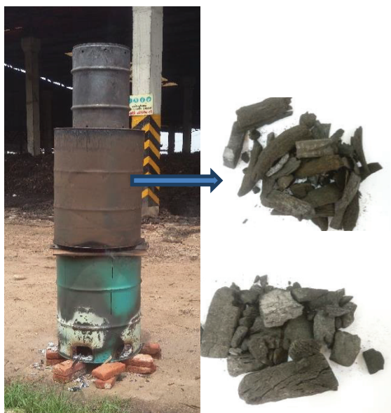
Figure 2- Biochar production technique (left) and the resulted MSW biochar (Top right) and wood biochar (Bottom right)
