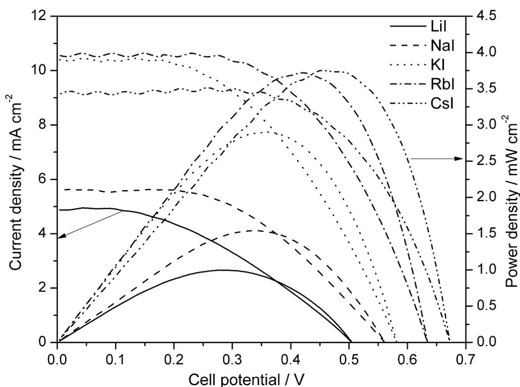
Fig. 7 Current density versus cell potential for the series of DSSCs containing the  $(AN)_{10}(EC)_{25}(PC)_{20}(MI)_{1.2}(I_2)_{0.12}$  series without additives.
