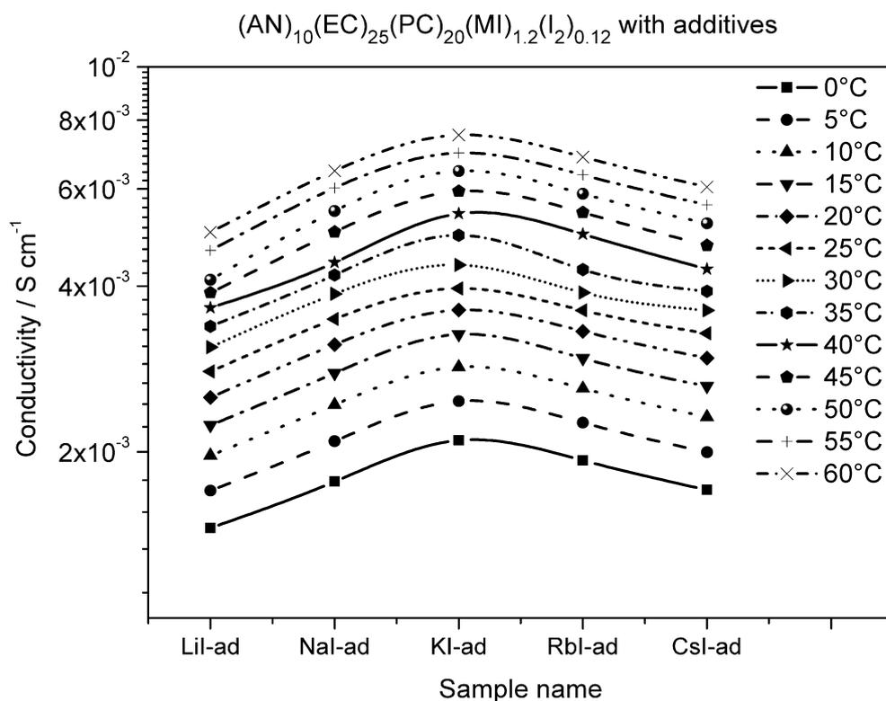
Fig. 4 Conductivity isotherms of the  $(AN)_{10}(EC)_{25}(PC)_{20}(MI)_{1.2}(I_2)_{0.12}$  series with additives Pr4NI, MPPII and 4TBP.
