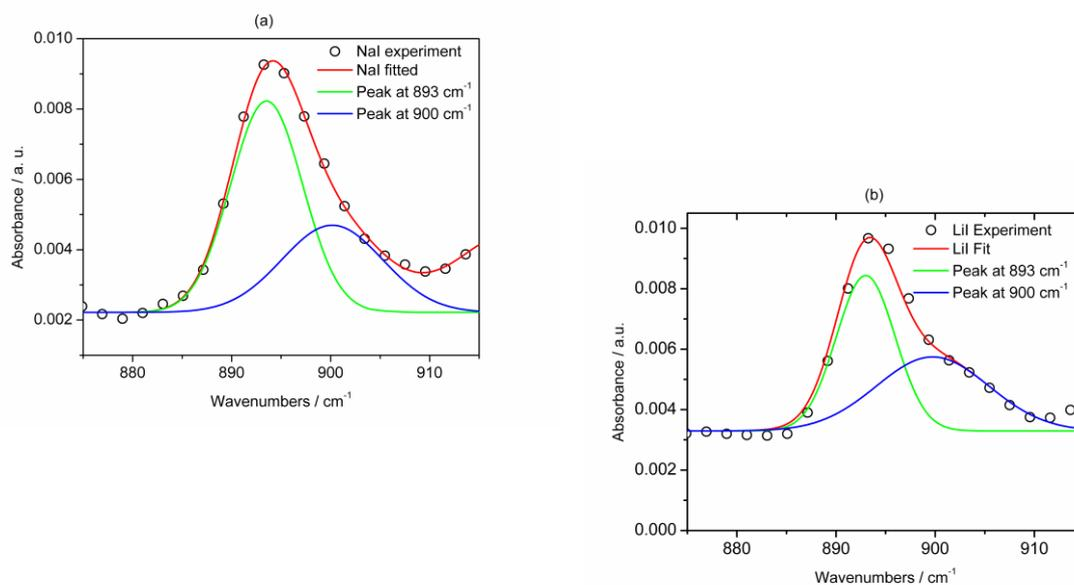
Fig 6 Curve fitting of the gel containing (a) NaI and (b) LiI. a) Peak position 893 and 900  $\text{cm}^{-1}$ , width 7.2 and 10  $\text{cm}^{-1}$ , area 0.05 and 0.03 (a.u.); b) Peak position 893 and 900  $\text{cm}^{-1}$ , width 5.4 and 11  $\text{cm}^{-1}$ , area 0.03 and 0.04 (a.u.)
