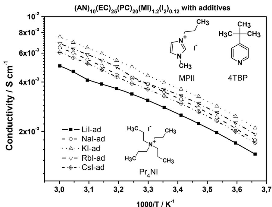
Fig. 2 variation of conductivity against inverse temperature ( $1000/T$ ) in the electrolyte  $(AN)_{10}(EC)_{25}(PC)_{20}(MI)_{1.2}(I_2)_{0.12}$  series with additives  $Pr_4NI$ ,  $MP11$  and  $4TBP$  (molecular formulas as insets) for different alkaline iodides.
