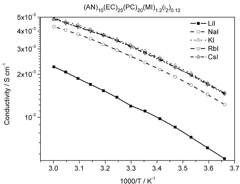
Fig. 1 variation of conductivity against inverse temperature (1000/T) in the electrolyte  $(AN)_{10}(EC)_{25}(PC)_{20}(MI)_{1.2}(I_2)_{0.12}$  series without additives for different alkaline iodides.
