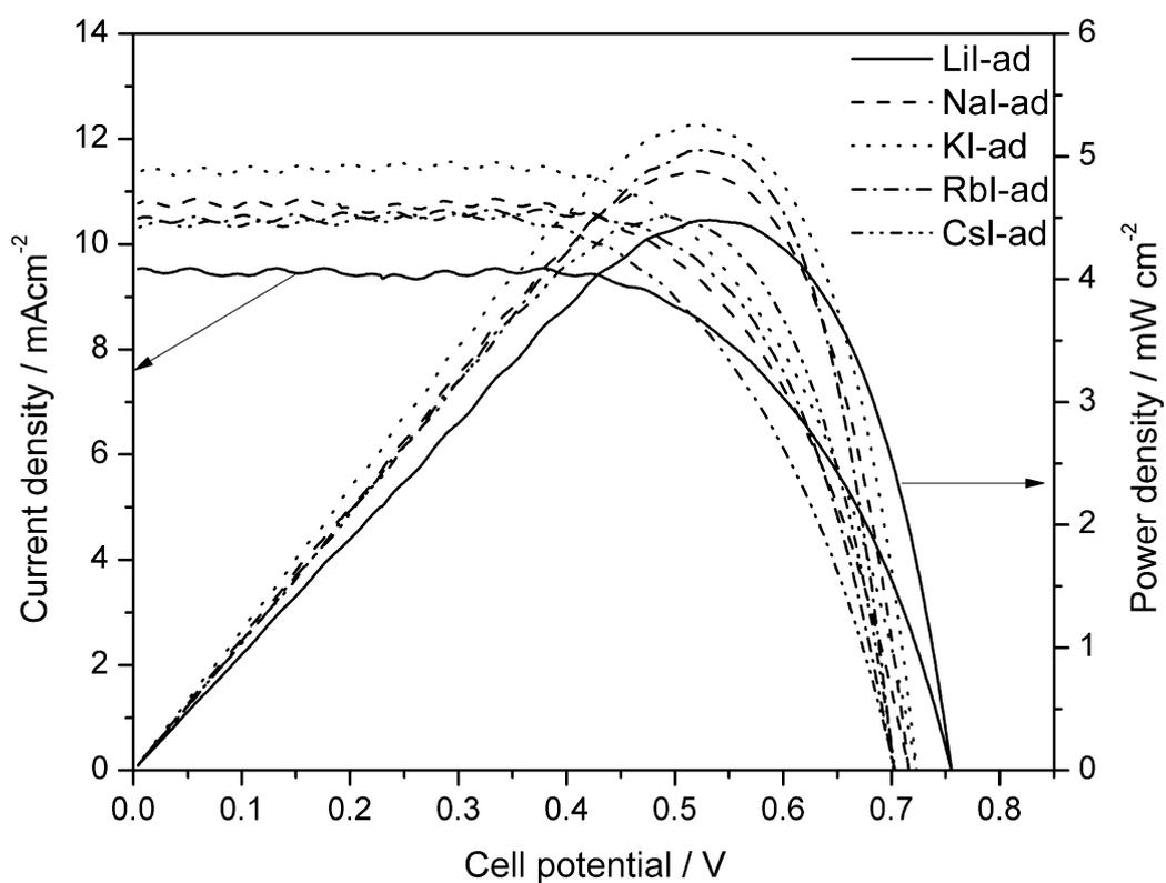
Fig. 8 Current density versus cell potential for the series of DSSCs containing the  $(AN)_{10}(EC)_{25}(PC)_{20}(MI)_{1.2}(I_2)_{0.12}$  series with additives.
