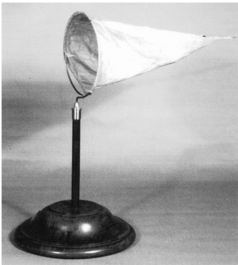
Faraday's Bag. Electric charge placed on a conducting body accumulates on the outside of the body. This can be demonstrated with a cloth bag mounted on an insulating stand. The cloth conducts well enough to allow the charge to travel from one surface of the bag to the other as it is turned inside out using the strings attached to both sides of the bag's vertex. This example is at the apparatus collection of Colby College. It is unmarked, but looks very much like an illustration in the 1860 catalogue of Edward S. Ritchie of Boston. The catalogue description is "Faraday's Muslin Bag; sustained upon an insulated ring of wire, with silk strings,...$4.00." (Photograph and notes by Thomas B. Greenslade, Jr., Kenyon College)
