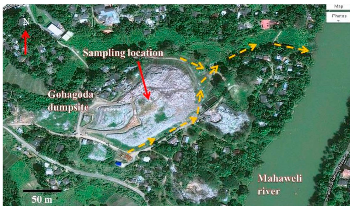
Figure 1. Schematic of the Gohagoda MSW dumpsite, the leachate sampling point at the top of the dumpsite and leachate drainage pathway (in yellow dotted arrows).
