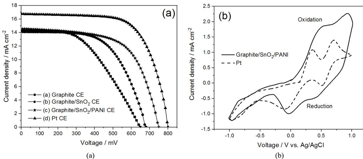
**FIGURE 2.** (a) Current density versus photo voltage characteristics of DSSCs with different CEs. (b) The cyclic voltammetry graphs of the graphite/SnO<sub>2</sub>/PANI composite CE, in a three-electrode arrangement using a 10 mV s<sup>-1</sup> scan rate.
