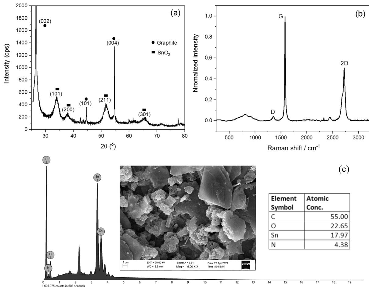
**FIGURE 1.** (a) XRD and (b) Raman spectra of graphite/SnO<sub>2</sub>/PANI composite material. (c) SEM surface image of graphite/SnO<sub>2</sub>/PANI composite CE and the EDS mapping graph by EDS spectroscopy (used with the permission of the SEM imaging facility of the Department of Geology, University of Peradeniya, Sri Lanka).
